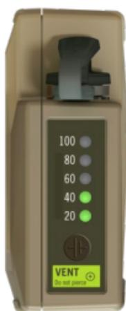
The SoloPack has an array of LED lights which indicate the capacity remaining in the battery by pressing the button. Each LED represents 20% remaining capacity meaning that five active LEDs indicate full charge. For example, two active LEDs indicate that the remaining capacity is greater than 20% but less than 40%, and so on. One exception to this rule applies when the remaining capacity is less than 10%: the bottom LED (next to the button) will blink upon pressing the button.
